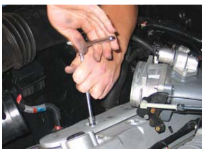
Swapping plugs on a Cobra is rather easy with the plug location in the center of the cam cover. For the passenger side, the inlet tube will require removal first, then it's just a few bolts to remove the coil-pack beauty cover.
