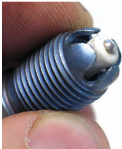
A close-up of the Brisk electrode and tip shows the deep ground electrode design that promotes spark discharge at the very tip of the plug. You can also see in this photo that the flame front would propagate in all directions. This means there is no need to index these spark plugs in the combustion chamber.
