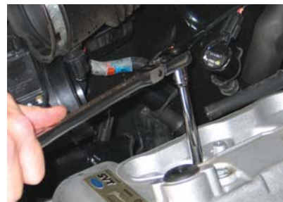
A standard 14mm plug socket and extension are all that's required to access the plugs. Make sure your plug socket has a strong rubber insert (a section of 3/8-inch hose will work in a pinch) to help pull the plug out of the depths of the cylinder heads.
