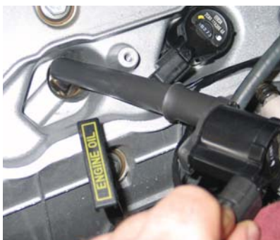
The coil packs are situated over the spark plugs and are easily removed with a twist and pull of the coil pack. You can leave the wiring harnesses connected and just lay the coil packs aside during removal of the plugs.
